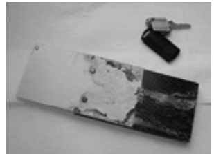
Fig. 1: Severe corrosion in aluminium/CFRP combinations after salt-spray test
