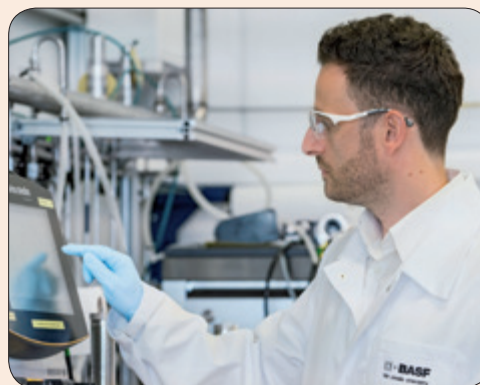
Fig. 8: A technician preparing a fermentation reactor for operation; keeping the conditions of the fermentation process adequate for optimum productivity of the respective microorganism is key to obtaining optimum performance (source: BASF SE).
