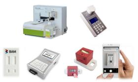
*Figure 1: Some portable immunoanalytical devices suitable for environmental monitoring (Top: Polarimeters for FPIA, Bottom: LFIA cassette with available reading devices).*
