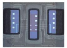
Figure 1: Microscope image of the packaged sensors chip (2.5 x 2.5 mm)
