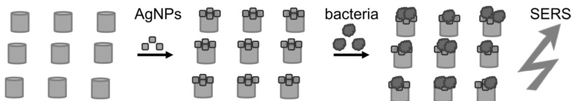
Fig. 1: Successive dielectrophoretic accumulation of silver nanoparticles (AgNPs) and of bacteria at nanoelectrode arrays, and bacteria detection by surface enhanced Raman spectroscopy (SERS).
