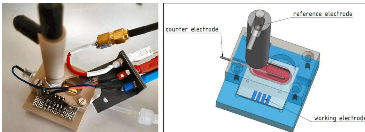
Figure 1: View and scheme of the measurement chamber developed and used for the investigations.
