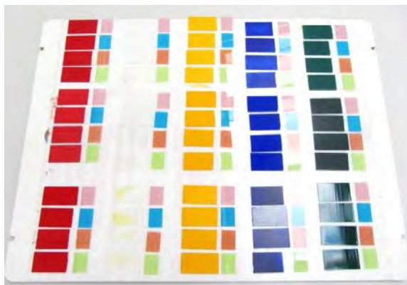
Figure 1: Self-made samples as this paint film used for the indoor ageing studies.
